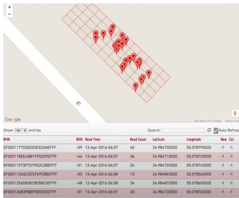
Figure 3. Vehicle location using RFID technology
