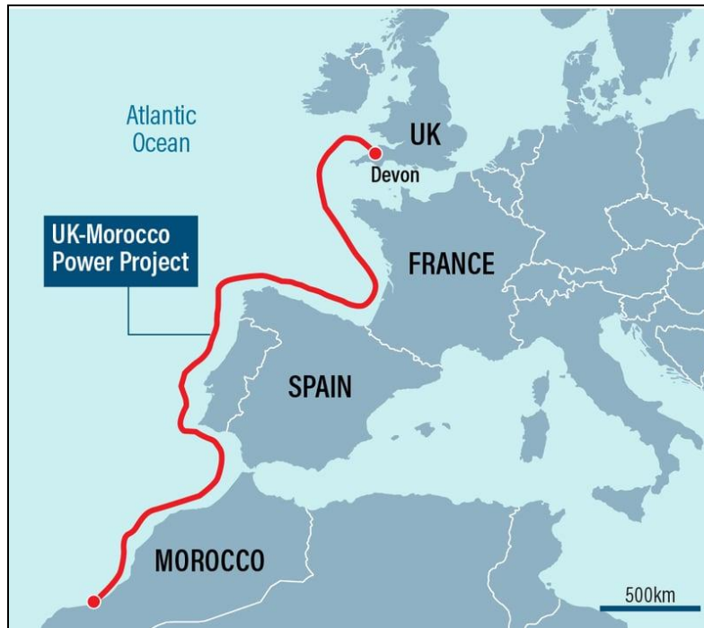
Figure 2. Morocco – UK Power Project Xlinks: visualization of the cable systems that will follow the shallow water route from the Moroccan site to a grid location in Great Britain.
