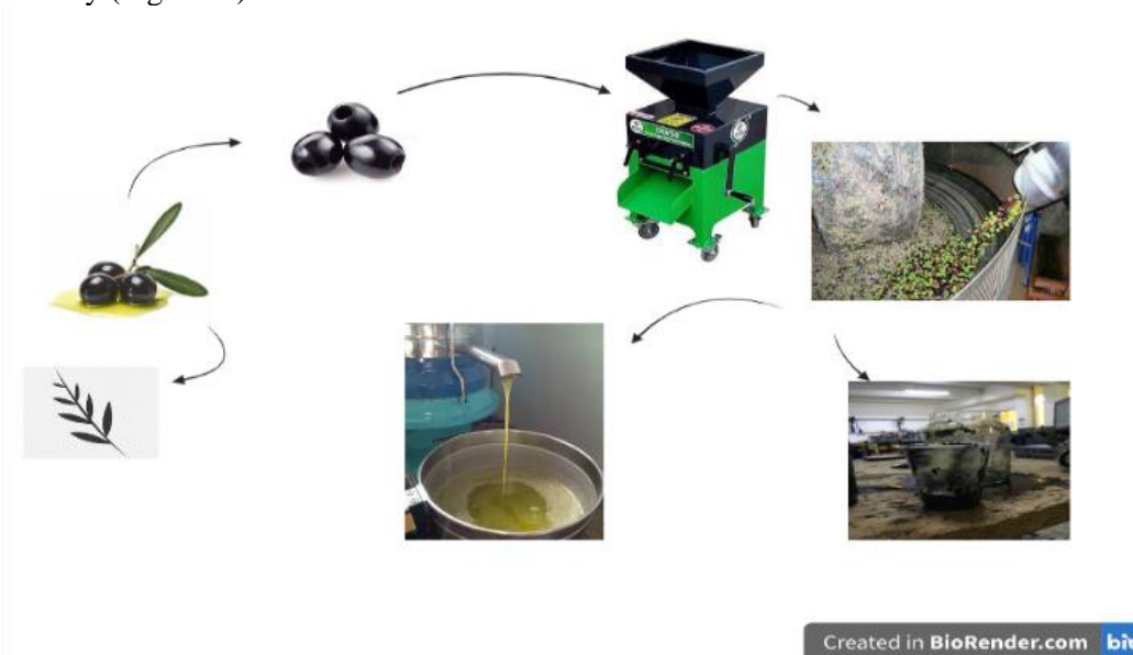
Figure 2. Olive processing process: Olive formation and growth, pouring into the hopper, taking it into the tank, squeezing, automation of separation, obtaining the residue
