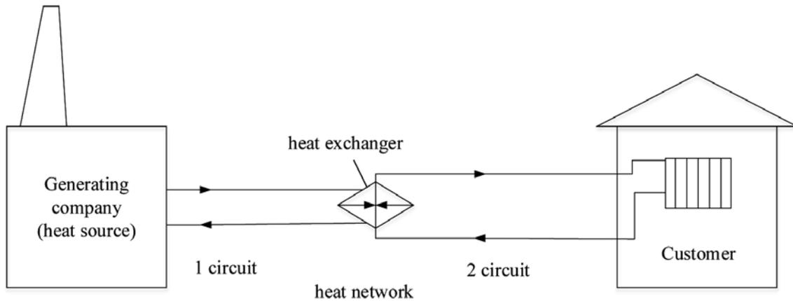
Fig. 7. Schematic circuit of an independent heat supply system
