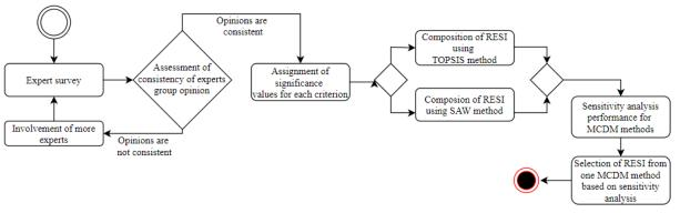
Fig. 1. RESI compilation algorithm
