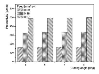
Fig 6. Dependence of production from feed and cutting angle of circular saw NOOK 450x50x2-z56 Source: authors.
