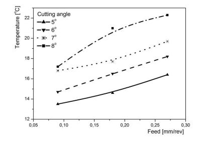
Fig 4. Dependence of temperature from feed and cutting angle of circular saw NOOK 450x50x2-z56 Source: authors.
