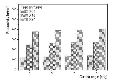
Fig 3. Dependence of production from feed and cutting angle of circular saw NOOK 200x50x1.5-36 Source: authors.
