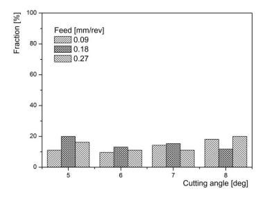
Fig 2. Dependence of fraction  $\leq 0.63$  mm from feed and cutting angle of circular saw NOOK 200x50x1.5-36 Source: authors.
